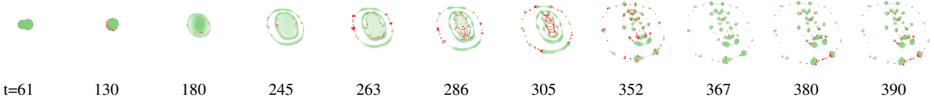
Fig. 11: Timesteps of the droplet dataset that were automatically selected by finding maxima of smoothed model error (cf. Fig. 12). High error locations are rendered in red. Several sparse important events are captured in the beginning: the initial collision, two disk separations, outer disk break-up. The rest of the timesteps correspond to a more chaotic mass separation phase of the data.
