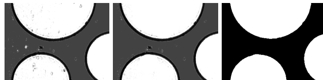
(a) original capture (b) manual cleaning (c) post-processing Figure 5: Mask pre-processing phases (zoom-in, Ca 1e-5, M 1 ).
